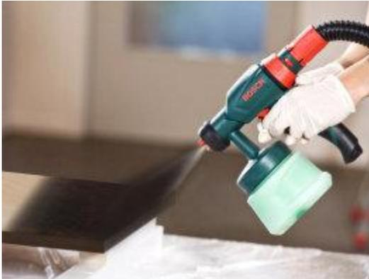
Staining refers to the process used to colour the wood. The wood stain can be applied with a fine spray system. After the stain has been applied, the surface of the wood remains unprotected until wax or paint/varnish is applied.
