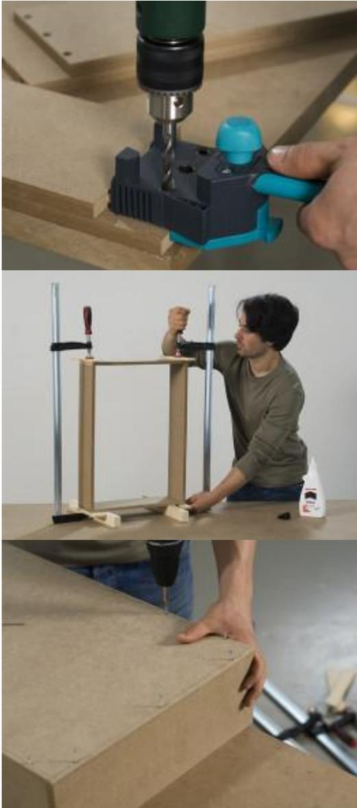
Of course, you can also fit the drawer sections using screws (3 x 25 mm). If you do so, follow the procedure described in the previous steps.
