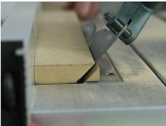
Cut two suspension rails (one for the rear panel and the matching piece for the wall) at a 45° angle from a board measuring 1050 mm in length and 120 mm in width. Adjust the saw blade of the circular saw to 45° and split the suspension rail board in lengths. Using the drill and 4-mm wood drill bit, predrill holes in the suspension rails and countersink the holes. Follow the same procedure for the spacer bars and the reinforcement panel.
