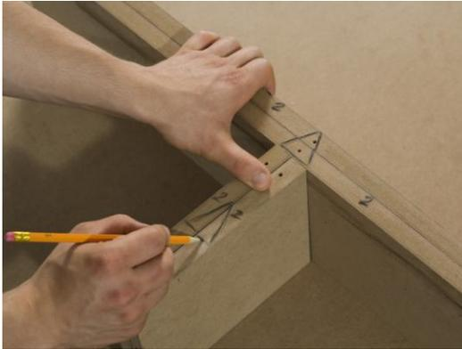
A shelf consists of two side panels enclosed by two shelf bases. Place the sections together in the way you want to assemble them and mark their respective positions using triangle symbols on the rear edges so that you always know what goes where at a later stage of assembly.
