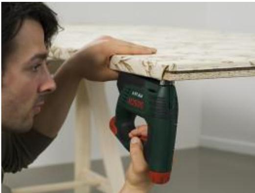
When cutting the fabric to size, make sure it is 60 mm wider and longer than the door leaf. Lay the fabric front side down so that it is smooth and place the door leaf in the centre of the fabric. Pull the fabric back towards you over the edges, fold it over twice and tack it in place on the back of the door leaf.
