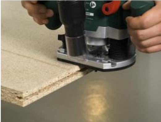
Using the slotting cutter, rout a groove that is 7 mm wide in the bottom edge of the door leaf. The groove is only 4 mm wide when you complete the first routing process. Adjust the routing depth by 3 mm and repeat the routing process: the groove is now 7 mm. Chamfer all edges of the door leaf by using a piece of sanding paper (grit of 120) at a 45° angle until a small bevel is created.
