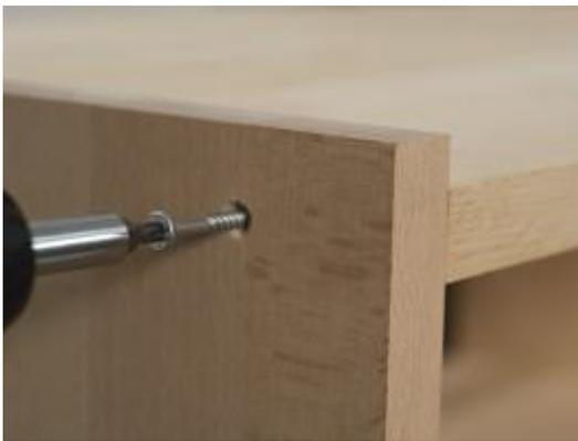
Once the gluing process is complete, insert the intermediate shelf base between the side panels that have been predrilled as required. (In our illustration, this is the right-hand compartment of the left-hand console section.) Secure the shelf base in place using the cordless screwdriver and screws (4 x 40 mm).
