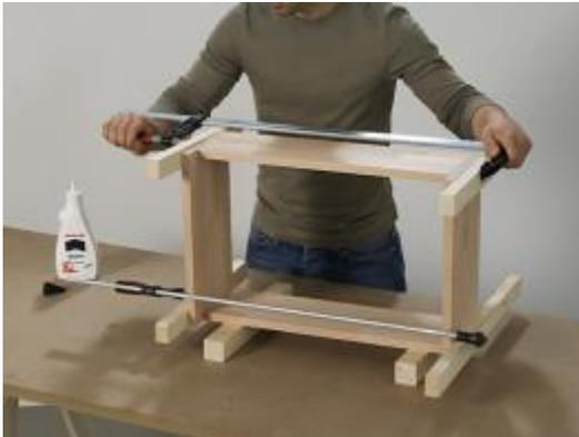
Dab glue into the dowel holes and the glue surfaces of the front and rear section and then insert the wooden dowels. After you have also applied some glue to the holes in the side panels, stick the front section, rear section and side panels together. Press the sections together using clamp clips. Refer again to the note on gluing in step 2.
