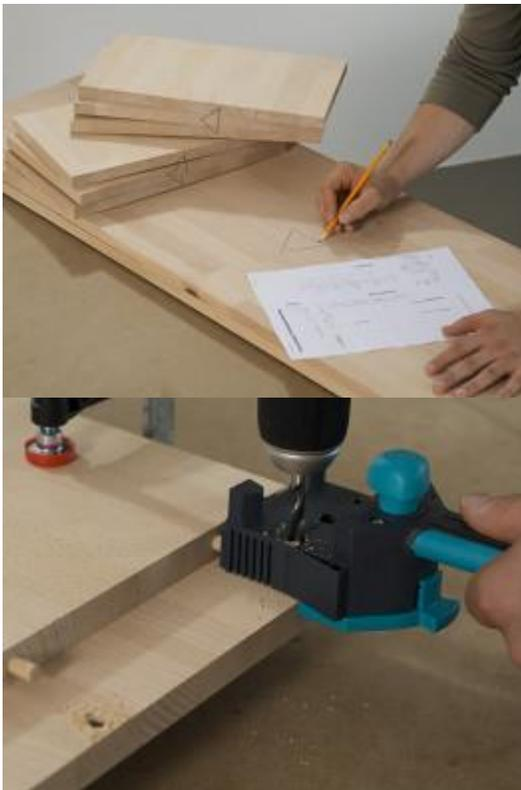
First, position the side panels and the top panel in the way you want to assemble them. Use a pencil to mark the positions on the rear edges of the sections so that you always know what goes where at a later stage of assembly.
