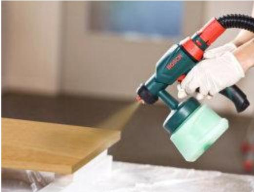
First read the manufacturer's safety and handling instructions thoroughly. Make sure the room you are working in is well ventilated and not used for smoking, eating or drinking. Generously apply the oil or wax with a fine spray system and remove any excess with a cloth. Observe the drying times specified by the manufacturer.
