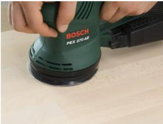
First chamfer all edges with sanding paper with a grit of 120 or 180 at a 45° angle to create a small bevel. Use your sander to sand all visible surfaces in the direction of the wood grain, first with coarse sanding paper (grit of 120, 180) and then with fine sanding paper (grit of up to 240).
