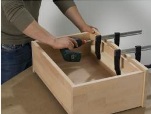
Pre-drill the base using the drill and 4-mm wood drill bit. Then fasten it to the front and rear section using screws (4 x 35 mm). Refer to the tip on screwing together two pieces of wood in step 3.
