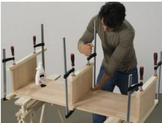
Apply glue to the dowel holes and the glue surfaces of the side panels and then insert the wooden dowels. Once you have also dabbed some glue into the holes in the top panel, join all the pieces together. Clamp the joints using clamp clips.
